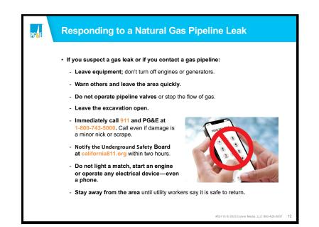
Responding to a natural gas pipeline leak. The single greatest risk from natural gas leaks is explosion. Even the smallest spark can ignite the gas, and sparks can come from some unexpected sources. So it's important to know the proper dos and don'ts for dealing with a natural gas leak.
